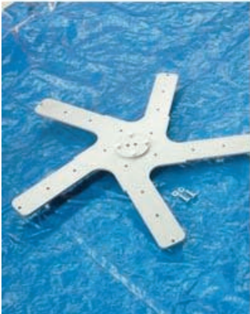
AFTER DISASSEMBLED BLADE SUPPORT, DISASSEMBLY HUB
